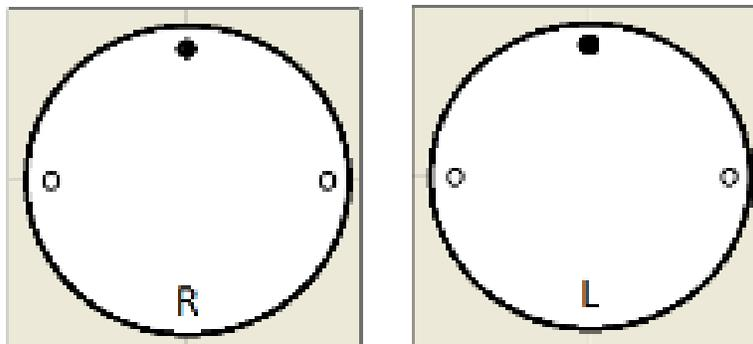
**Image 1:** Ampleye® laser marks at 3 & 9 o'clock, along with R/L to signify which eye the lens is made for. A black dot was placed 180 degrees from the R/L to signify how the lens should be oriented upon insertion.
