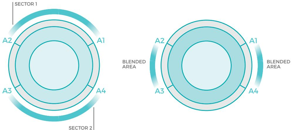
Record angles counter-clockwise around the lens as A1, A2, A3 & A4.
